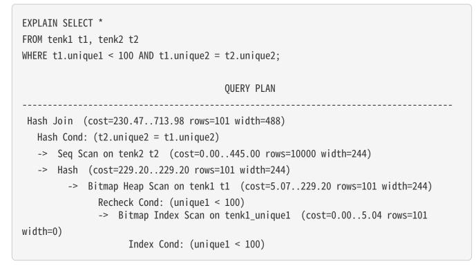
Here, the planner has chosen to use a hash join, in which rows of one table are entered into an in-memory hash table, after which the other table is scanned and the hash table is probed for matches to each row. Again note how the indentation reflects the plan structure: the bitmap scan on **tenk1** is the input to the Hash node, which constructs the hash table. That's then returned to the Hash Join node, which reads rows from its outer child plan and searches the hash table for each one.
