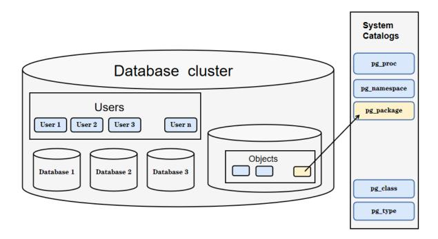
The yellow color in the diagram shows the new modules added by IvorySQL on top of existing PostgreSQL while IvorySQL has also made changes to existing modules and logical structures as well.
